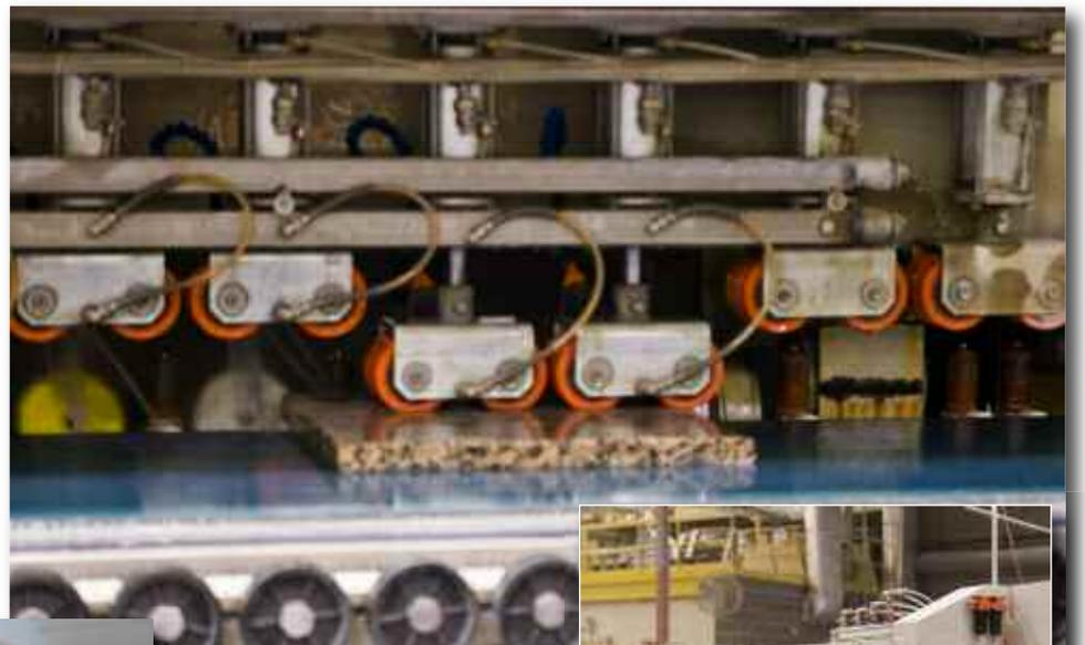
Above: Commandulli Omega 100 Line Polisher applies an edge treatment to a vanity tops using SuperEdge Wheels. Preston also uses Toro wheels on this machine for flat edge polishing
